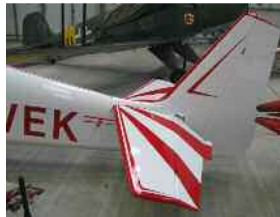
Finding a fibreglass fin fillet to fit was one of many challenges
