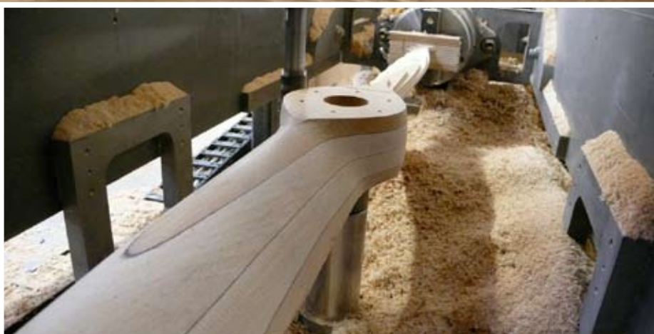
Use of numerically-controlled machinery at Hercules ensures that the production item conforms with the computer model. Very little hand-finishing is required, such is the precision (inset photo)
