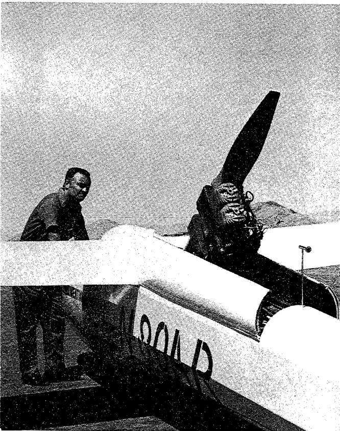
Bill Mouton demonstrates the ease of extending his Hirth engine on the SF-27M. The crank in the cockpit only requires 3\frac{1}{2} turns to fully extend or retract the engine. Bill now has an electric starter in his ship.
