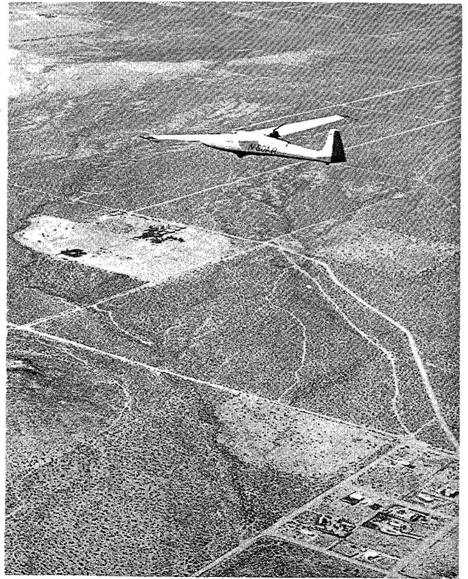
SF-27M with engine halfway retracted in flight.
