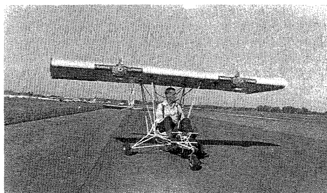
Photo 5—N11V—a true single-place Breezy, Jr. with only 14-foot wingspan and gross weight of 340 pounds, (with semi-fly-weight pilot-designer-builder, Wilbur Staib). Two 8.2-cubic inch (Chrysler) West Bends and Troyer 24-12 props, these being tractors instead of pushers. With near 100 pounds static thrust would get off rather quickly on hard surface. EAA Fly-In, Rockford, Illinois, August 1966.
