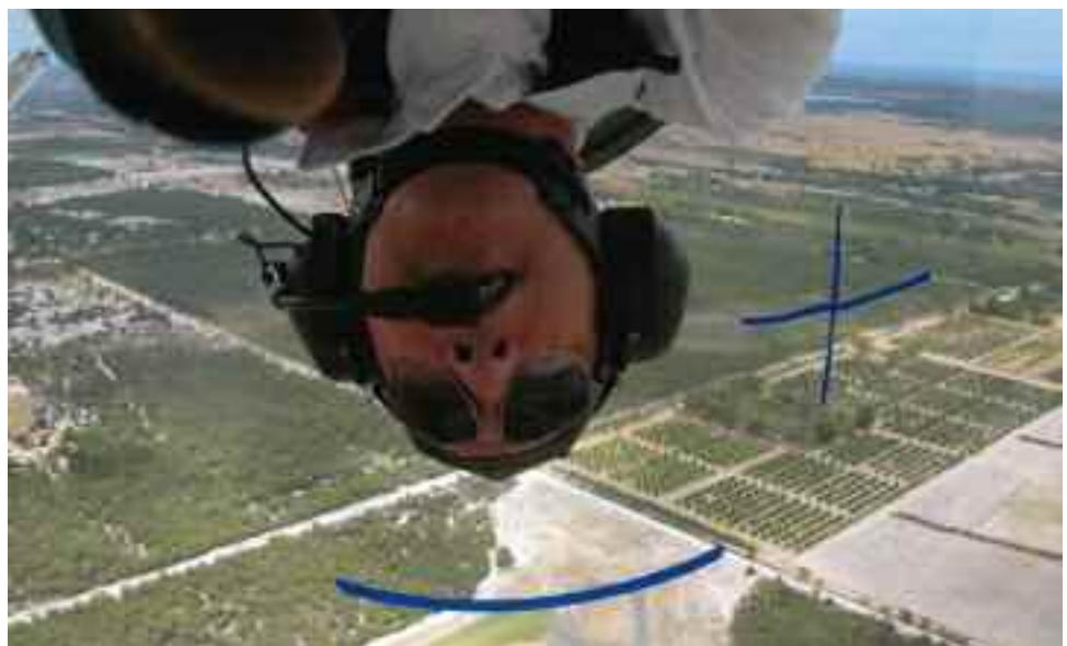
Coloured tape stuck to the inside of the canopy can be used to mark the inverted horizon or an accurate 45 degree line
